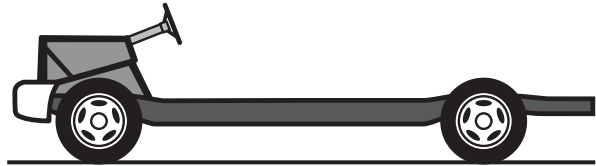
Stripped Chassis: Choice of 138.0", 158.0" or 176.0" Wheelbases
