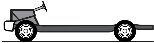
Stripped Chassis: Choice of 138.0", 158.0" or 176.0" Wheelbases
